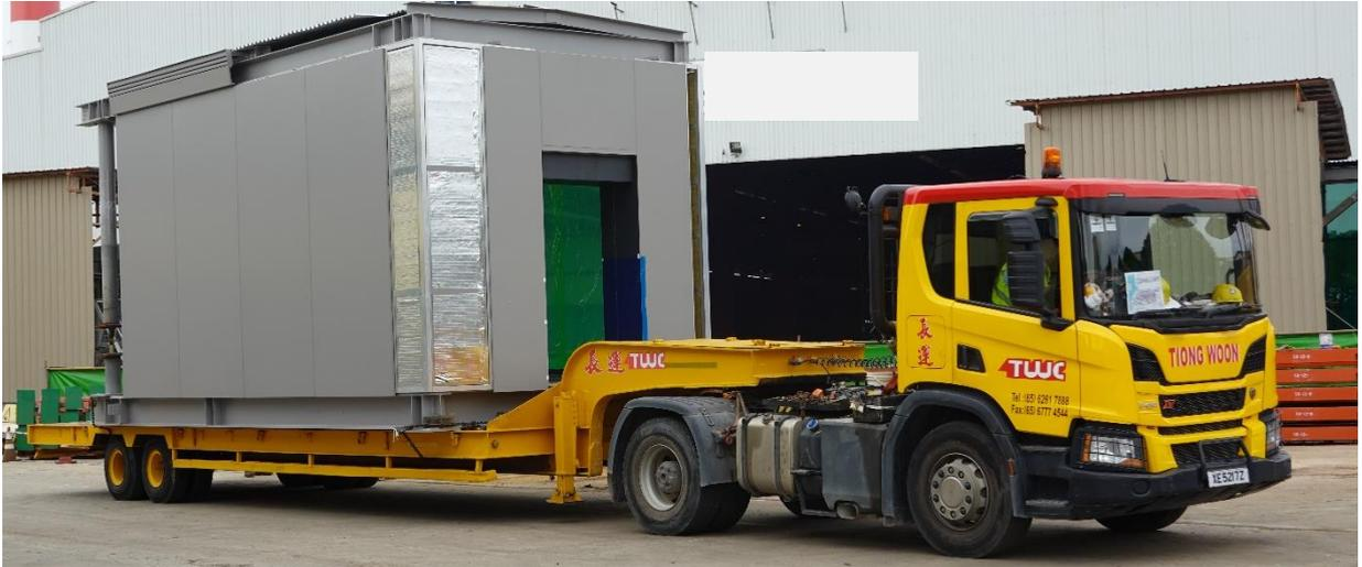
Measuring 21.42m (L) x 3.28m (W) x 4.3m (H) & weighing 52.6 Tons for the longer frame, 7.76m (L) x 3.7m (W) x 4.2m (H) & weighing 19.4 Tons for the shorter frame, we deployed a 12-axle Cometto connected to a Prime Mover to transport the longer frame. A Prime Mover with a Low Bed Trailer was deployed to transport the short frame.
